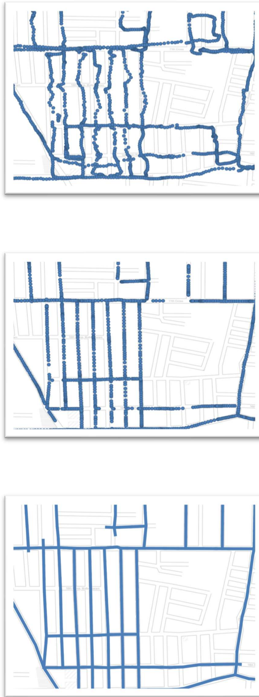
Figure 19 (top panel) Raw GPS measurements; (middle panel) snapped GPS measurements; (bottom panel) gridded road segments.
